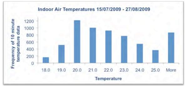
Figure 9: Chart showing indoor air temperature ranges in June/July 2009
